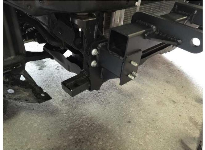
Install the Mobtown Recovery Bar onto the studs from which the crash bar supports were removed. Reuse (3) nuts per side from the crash bar supports. Note: The studs may need to be bent back into alignment. Use a rubber mallet to gently tap them straight so the Recovery Bar slips on all (6) studs smoothly.
