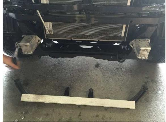
Remove (3) nuts from each side of the front crash bar. This will allow removal of the crash bar from the rectangular aluminum supports. The crash bar will be reused.
