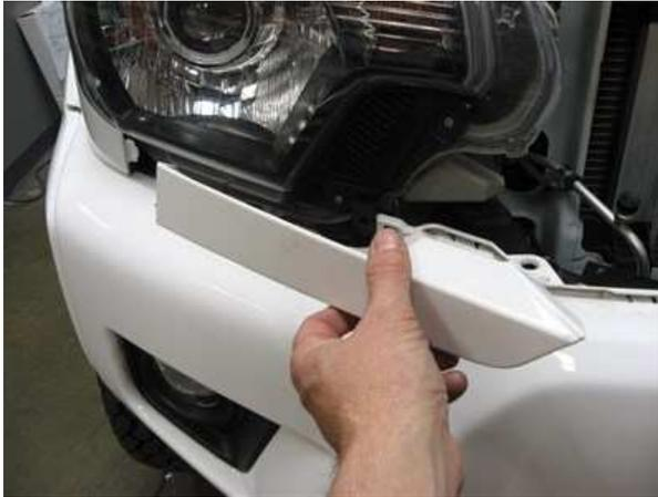
Remove plastic filler panel under headlight. The filler panel has a plastic clip on the backside. Once unclipped the filler will slide out. Be careful to pull straight or the filler panel will break.
