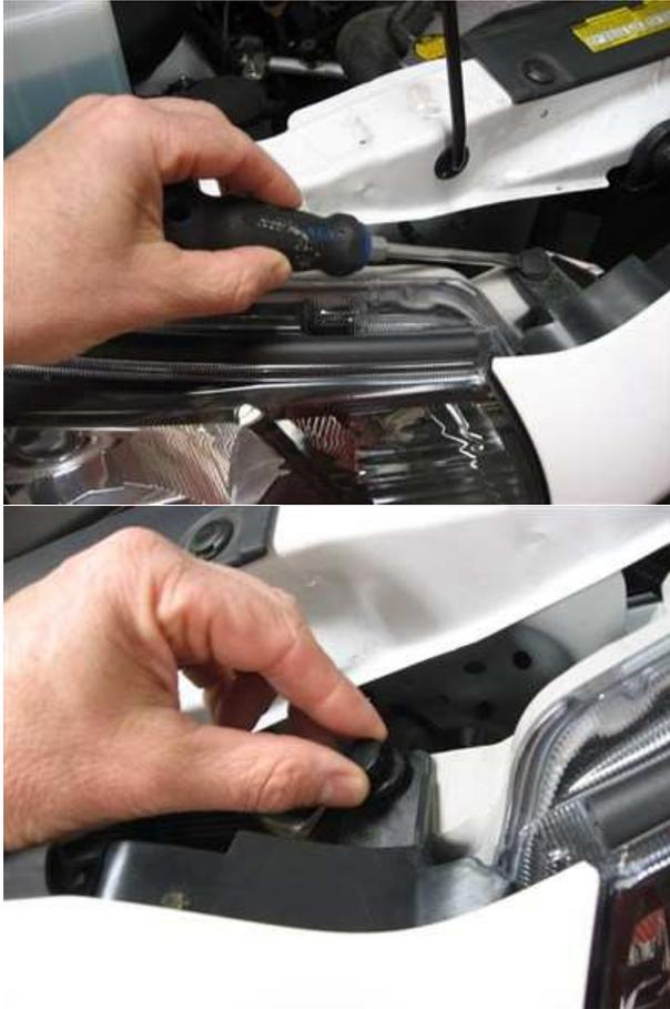
Use a screwdriver to unclip the push clips along the top of the grille. Remove clips from grille.
