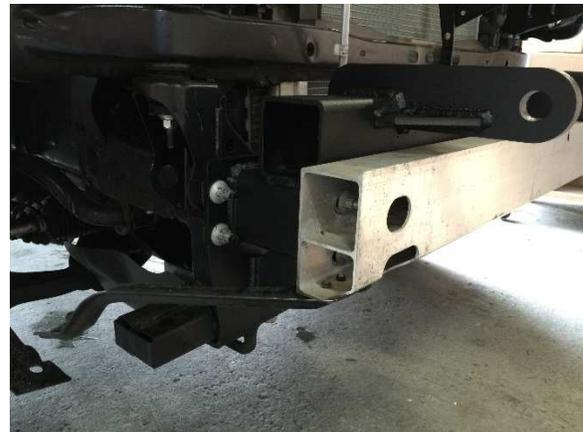
Reinstall the crash bar (not including the supports) onto the studs in the front of the Recovery Bar. Reuse the remaining nuts from the crash bar.
