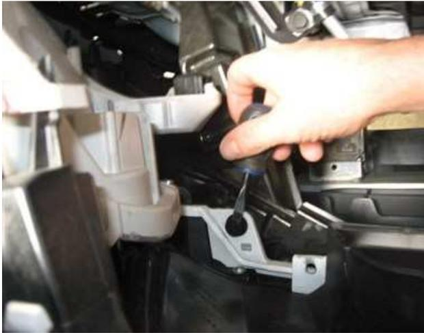
Remove the plastic clips along the top of the bumper cover
