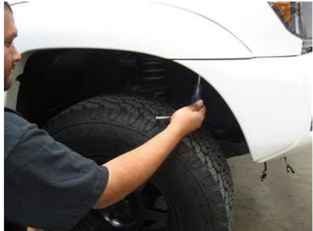
Remove the bolt located in the front section of the fender well as shown.
