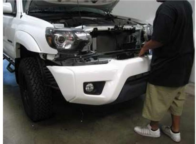
Remove the bumper from the vehicle. Make sure to unclip fog lamp wiring harness if necessary.
