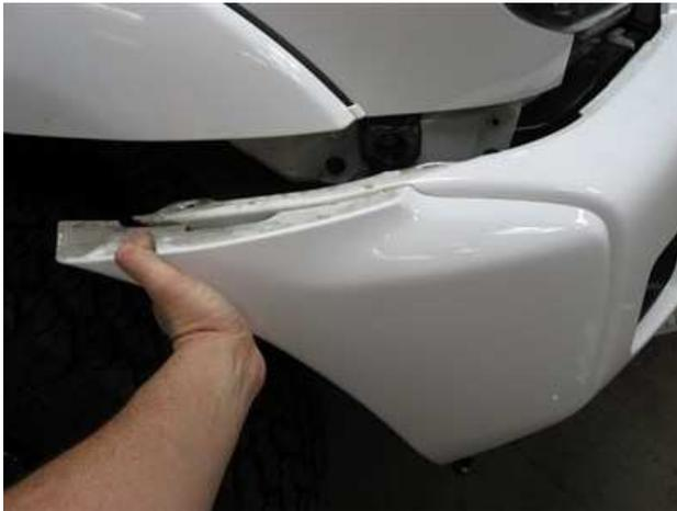
The bumper cover will release from the clip by pulling away from the vehicle.
