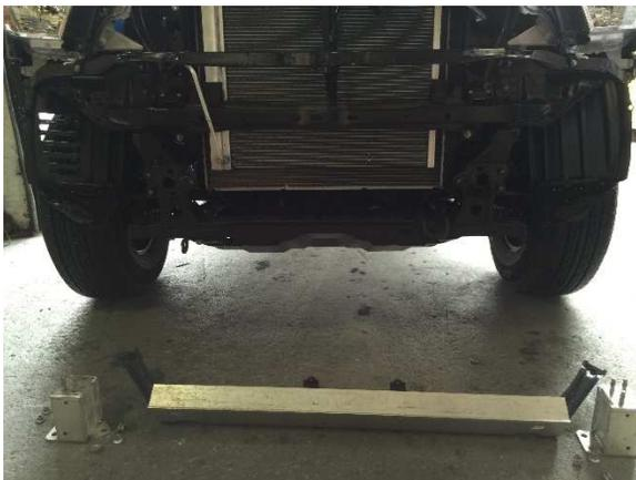
Remove both aluminum crash bar supports by removing the nuts and sliding it off the studs.
