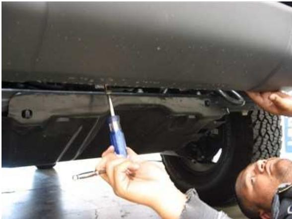
Remove bolts along the front underside of the bumper.
