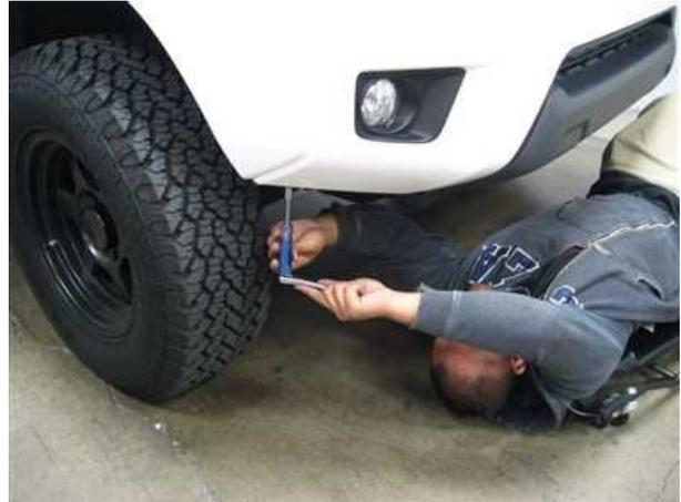
Remove the bolts on the right and left underside of the bumper.
